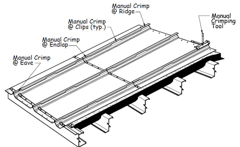
Before beginning, ensure that the panel is installed correctly and is free of all debris and contaminants such as sand, snow, excessive fluids, sealant/mastic, tools, extensions cords, etc... Also, always attach a safety hook to a tether during any time the seamer is on the roof to prevent it from falling off.
