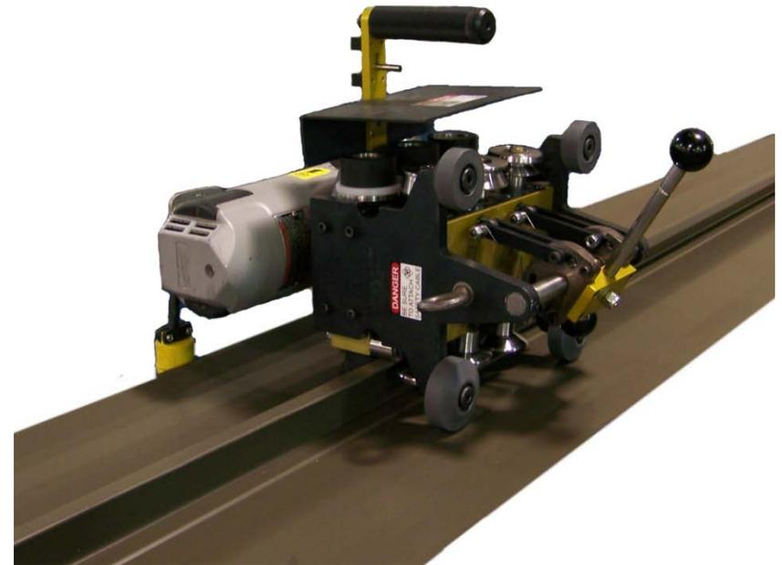
It is important to remember to use extreme caution when reaching the edge of the roof. Stop the seamer while the wheels remain on the roof panel. Roll machine back to a safe working area before disengaging the locking handles.
