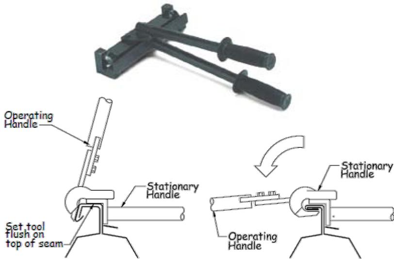
Next, place the machine on the hand crimped portion and engage the locking handle by pulling out until the handle locks into place. Add the power supply into the pigtail plug near the handle of the machine and turn the machine on. Run the seamer for about 12" to ensure that you are receiving the desired seaming operation. If so, continue in this manner for the completion of the run. If not, STOP SEAMING and contact Technical Support immediately.
