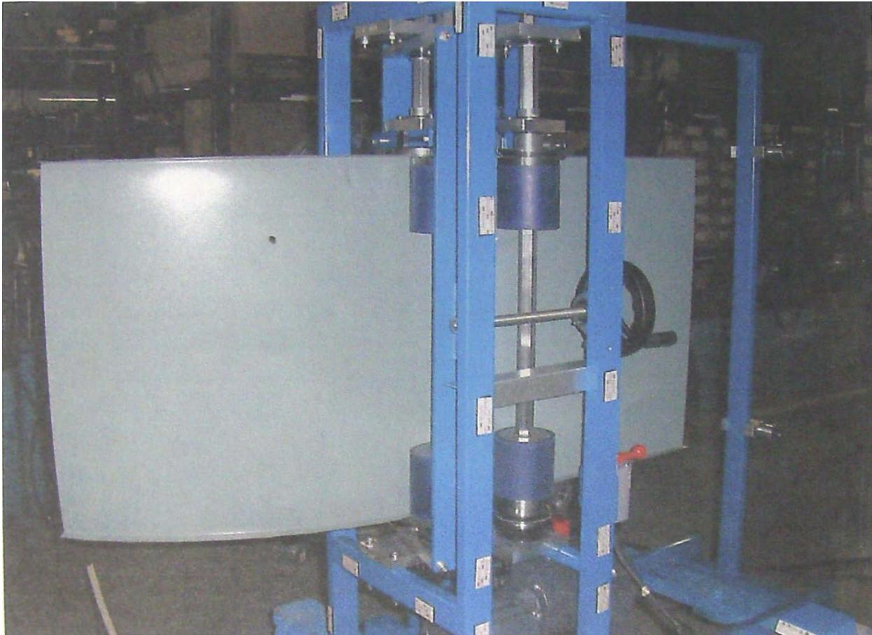
The AEP Span Select Seam<sup>®</sup> Curving Machine is designed to curve both the roof panels and the narrow batten caps. The amount of radius possible will vary with the material type and material thickness. The user will not be able to obtain the same minimum radius with different materials. The best results will be obtained by using the referenced scale on the machine to develop a "log book" of radius sizes depending on the type of material type and material thickness.
