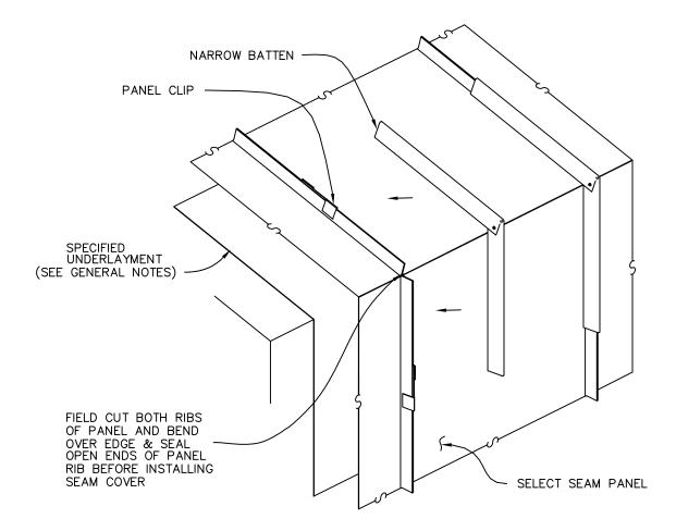
DESIGN CAUTION: TURNING PANELS DOWN FOR FASCIA MAY ESTABLISH UNWANTED POINT OF PANEL FIXITY. DESIGN NOTE:
