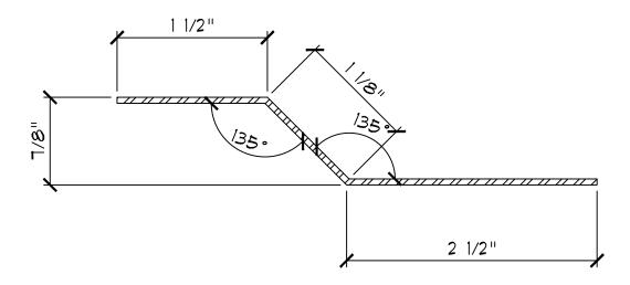
HIGH 16ga SUPPORT W/ INSULATION 33 KSI MIN. (USED WITH SPAN LOK 3" PANEL CLIP
