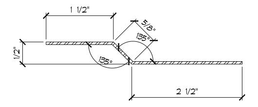
LOW 16ga. SUPPORT W/ NO INSULATION 33 KSI MIN. (USED WITH SPAN LOK 2 1/2" PANEL CLIP)
