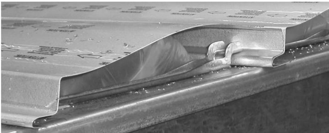
24ga PS-12 Panel at 100psf test point (138psf max obtained)
