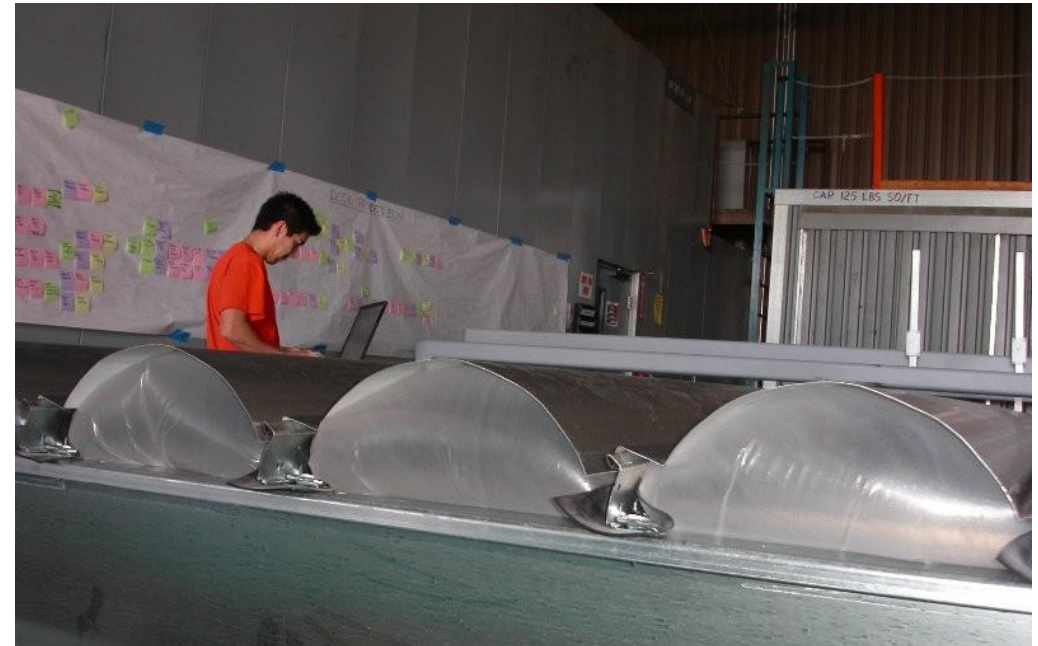
Uplift Panel Testing
