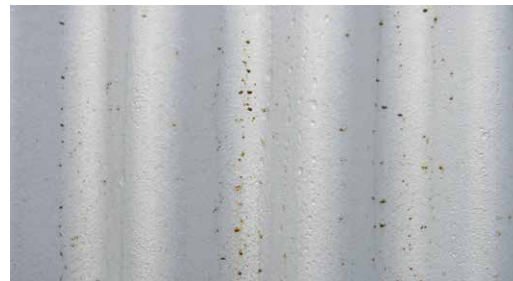
Moderate swarf staining on ZINCALUME Plus.
