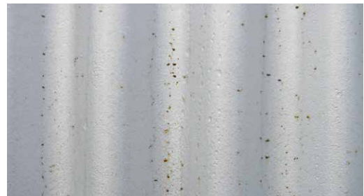
Moderate swarf staining on ZINCALUME Plus.
