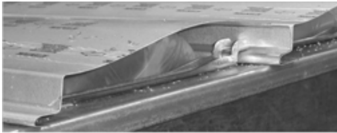
24ga PS-12 Panel at 100psf test point (138psf max obtained)
